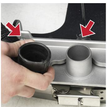
**1** Check if the suction hose is correctly installed and clean.
