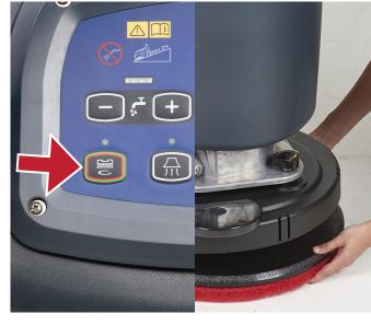
12. Press the click-off button and wait for the brush/pad holder to fall on the floor. Remove to clean or change brush.
