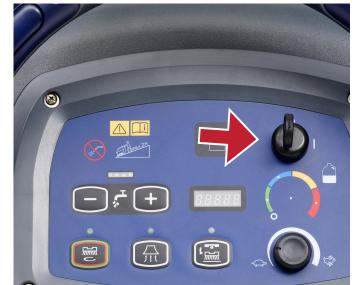
6. Lower the brush deck with the pedal. 7. Turn on the key, then slightly press the handle switch to engage the brush.
