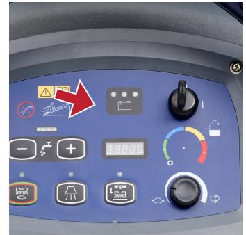
2 Check if there isn't any brush motor 3 overload i.e. 3 LED lights flashing simultaneously.
