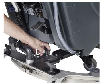
3. If the squeegee is not connected to the machine: install and fasten it with the handwheels, then connect to the suction hose.
