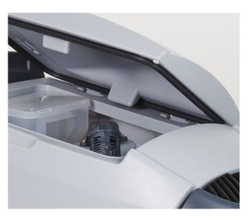
18. Park the machine with the recovery tank cover open.
